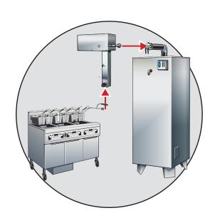
The WOPS System is an ideal way to move fats, oils, and grease from food service equipment to the containment tank when there is no built-in filtration pump.
